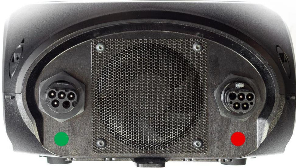
4] To unlock the cables, first turn off the power. Use a flathead screwdriver to unlock the latch [see figure]. Pull on the plug, leaving the latch unlocked. To reconnect the cable, a screwdriver is not necessary. Do not rotate the plugs while connecting the cable.
